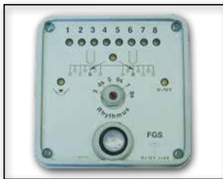
The FGS tramlining system switches and regulates the tramlines. Manual correction to the tramline position is provided as standard. An optional tank reserve indicator can be integrated.
