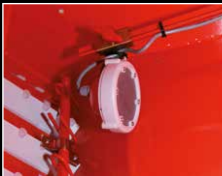
The tank reserve indicator is height adjustable
